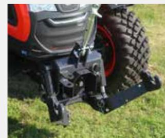
**FRONTKRAFTHEBER UND -ZAPFWELLE**
